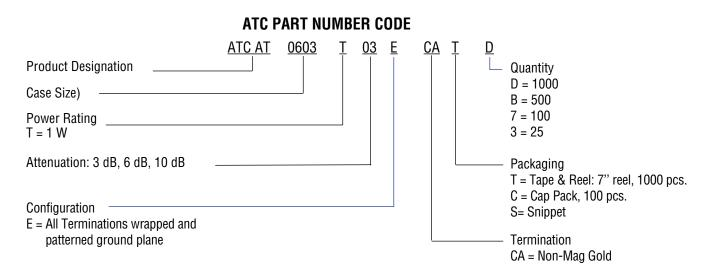
The above part number refers to an ATC AT 0603 Case Size with an attenuation of 3dB, 1W Power Rating, wrapped and patterned ground plane configuration with Non-Mag Gold Termination and tape and reel packaging, 1000 pcs.
