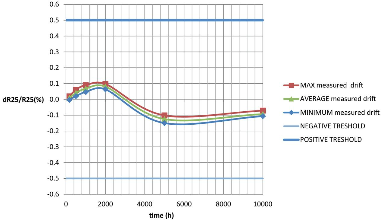
Fig. 1 - R<sub>25</sub> °C Drift after Storage at 125 °C for 0603 Case
