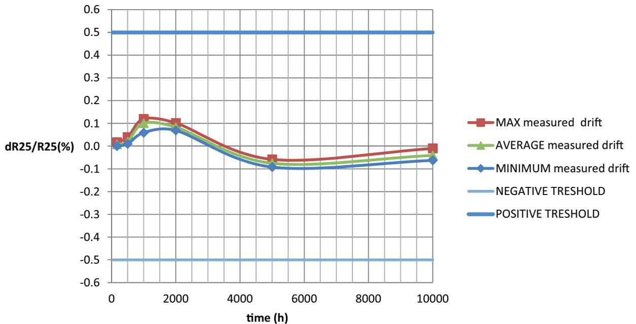
Fig. 2 - Drift in Storage at 125 °C for 0402 Case
