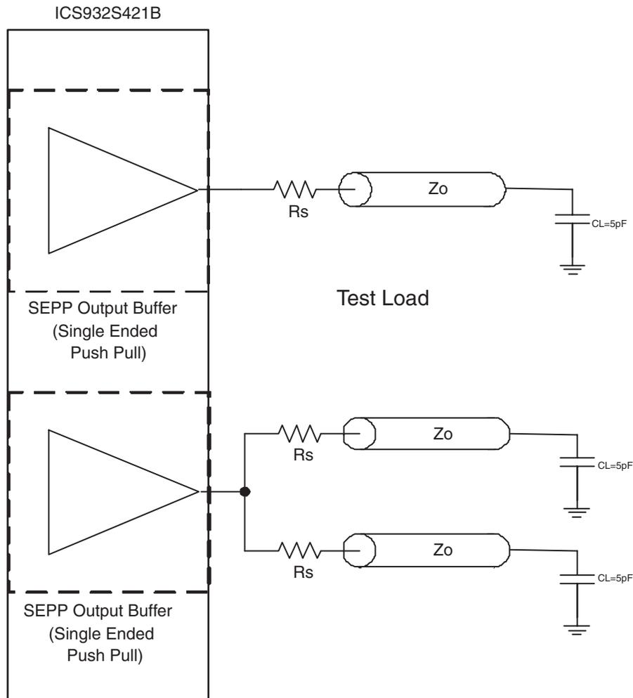
The singled-ended outputs of the ICS 932S421B default to a drive strength of 2 loads. The REF clocks can be turned down to 1-load strength via the SMBus. Suggested termination resistors are as follows for transmission lines with  $Z_o = 50$  ohms:
