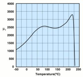
Measured on an 18/10/6mm toroid at 100kHz.
