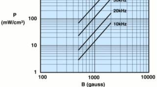
Measured on an 18/10/6mm toroid using the Clarke Hess 258 VAW at 100°C
