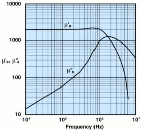
Measured on an 18/10/6mm toroid using the HP 4284A and the HP 4291A.
