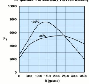
Measured on an 18/10/6mm toroid at 10kHz.
