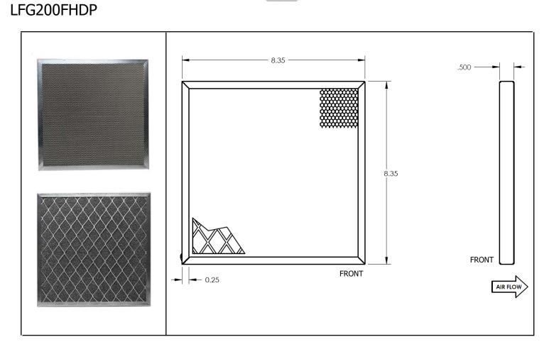
Orion Fans Pyrocide filters meet stringent flame safety standards for fire containment in electronics enclosures by preventing flames from propagating through the vent panels. The pyrocide coating has an ASTM E-84 Class A rating with low flame spread and low smoke index values. A thin coating in the honeycomb cells reacts on exposure to flame and expands rapidly, to prevent flames from propagating through the vent panels.
