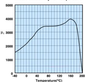
Measured on a 17/10/6mm toroid at 10kHz.
