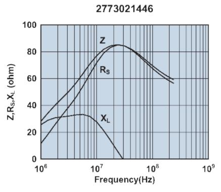
Impedance, reactance, and resistance vs. frequency.
