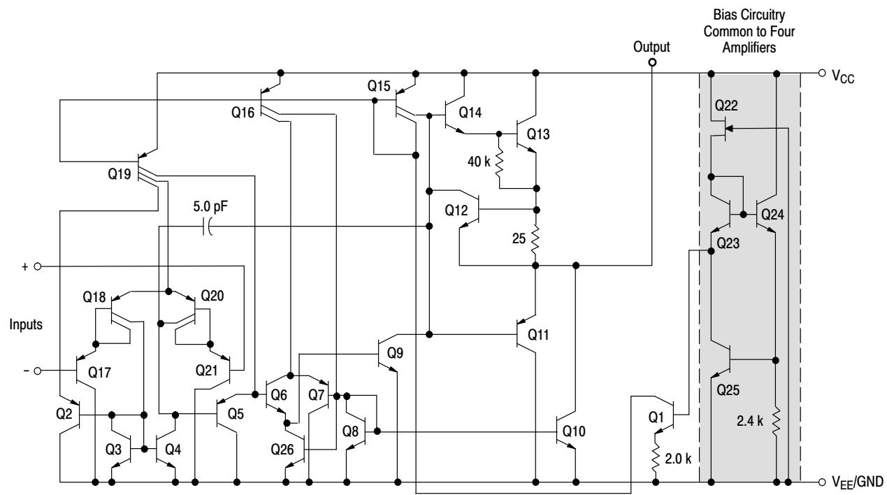
**Figure 1. Representative Circuit Diagram**
