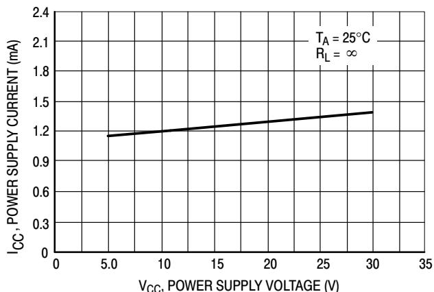
**Figure 9. Power Supply Current versus
