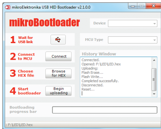
Figure 3-8: mikroBootloader ready for next job
