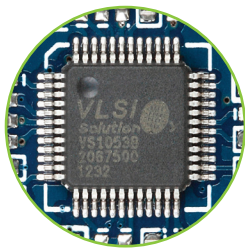
Figure 8-1: On-board VS1053 MP3 codec
