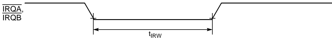
Figure 10-7 External Interrupt Timing (Negative Edge-Sensitive)
