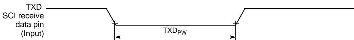
Figure 10-18 TXD Pulse Width
