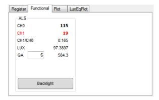
The Ch 0 and Ch 1 photodiodes output values are shown, and their ratio is shown below.
