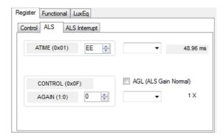
ATIME Register (0x01) controls the ALS integration time. The actual time is:
