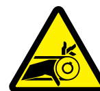
W3154 Belt Drive Entanglement Hazard
