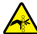
W3153 Pinch Point Hazard
