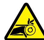
W3154 Belt Drive Entanglement Hazard
