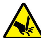
W3158 Cut or Sever Hazard
