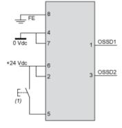
(1) Restart With External Device Monitoring (EDM) feedback loop
