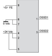
With External Device Monitoring (EDM) feedback loop
