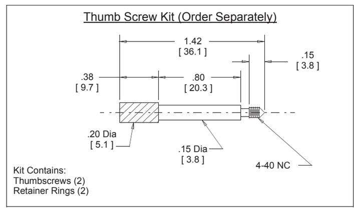
Note: The 3M™ 3341-7 Thumb Screw contains lead in the base material, therefore RIA E5 & C3 apply when using this hardware.
