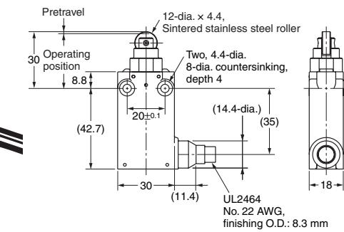
**Roller lever (Metal lever, resin roller)**
