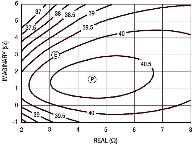
**Figure 8. P1dB Load Pull Output Power Contours (dBm)**
