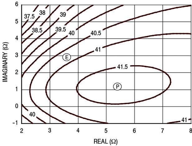
Figure 12. P3dB Load Pull Output Power Contours (dBm)
