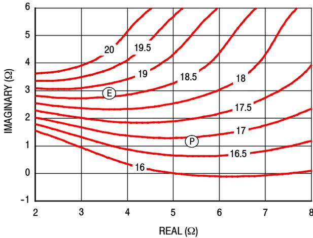
Figure 14. P3dB Load Pull Gain Contours (dB)
