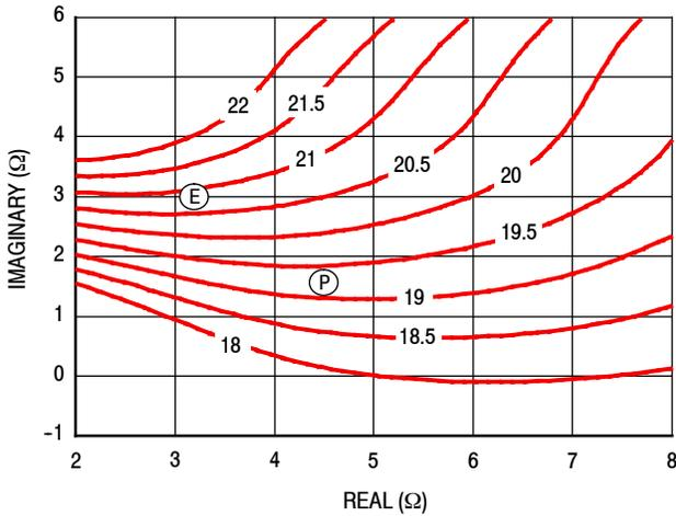
**Figure 10. P1dB Load Pull Gain Contours (dB)**
