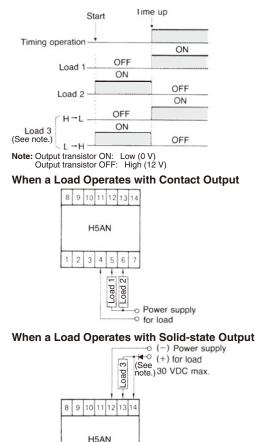
Note: Connect a diode when using a Power Supply of 12 V or less.
