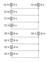
4. When changing the set time while power is being supplied, an inadequate push of the thumbwheel switches will display two numbers in one digital display window, causing the operating time to drift widely. Therefore, press the thumb-wheel switches surely. Take particular care in the case when the other three digits are all zero, since the improper setting of the fourth switch to create four zeroes will cause a momentary output.
