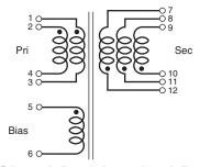
Primary windings and secondary windings to be connected in parallel on PC board.
