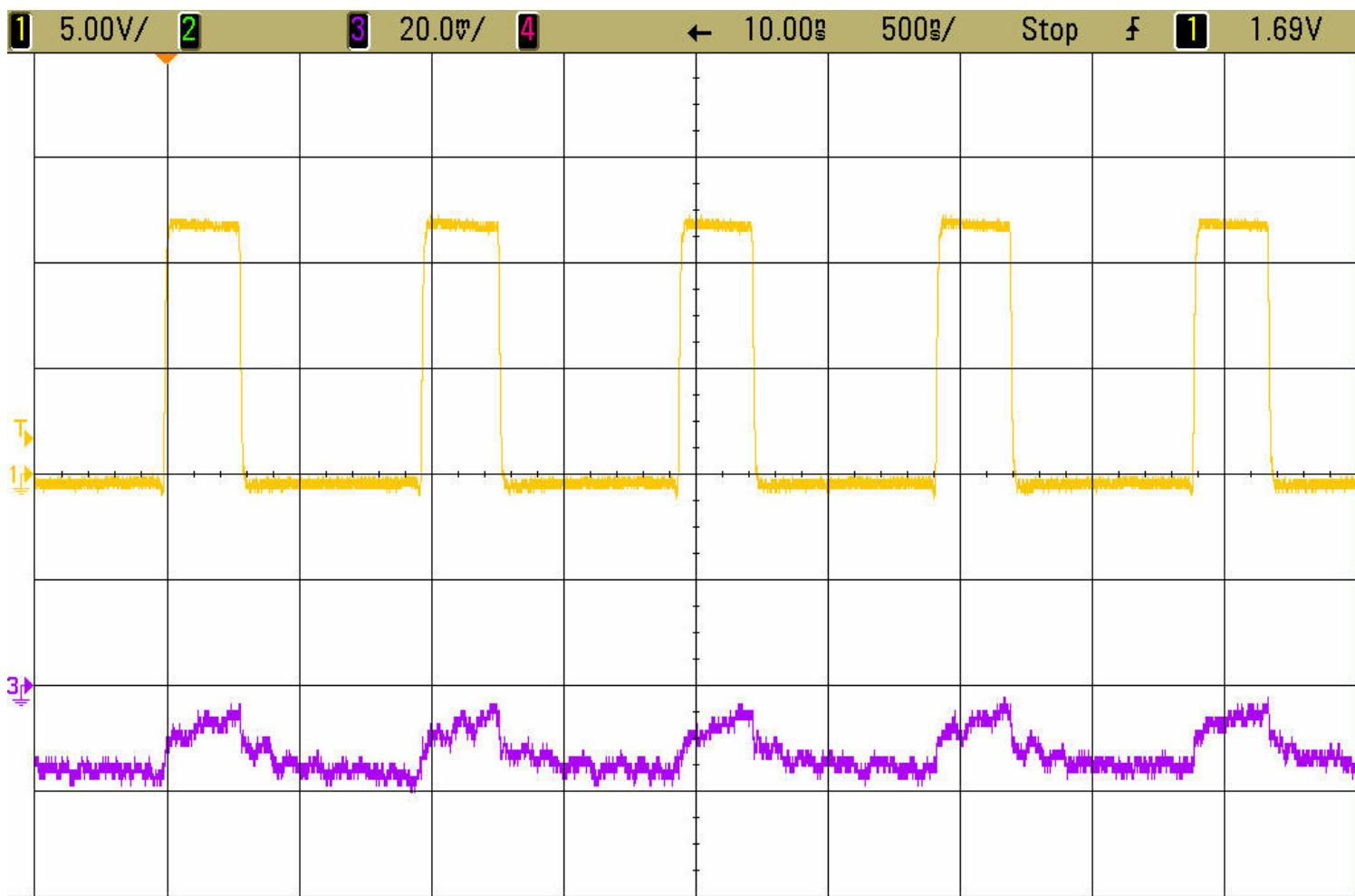
**Figure 3. Switch Waveform & Output Ripple Voltage**
