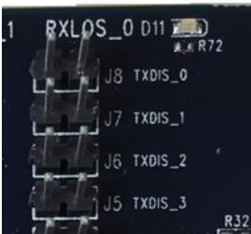
←Headers to manually enable the transmitters
