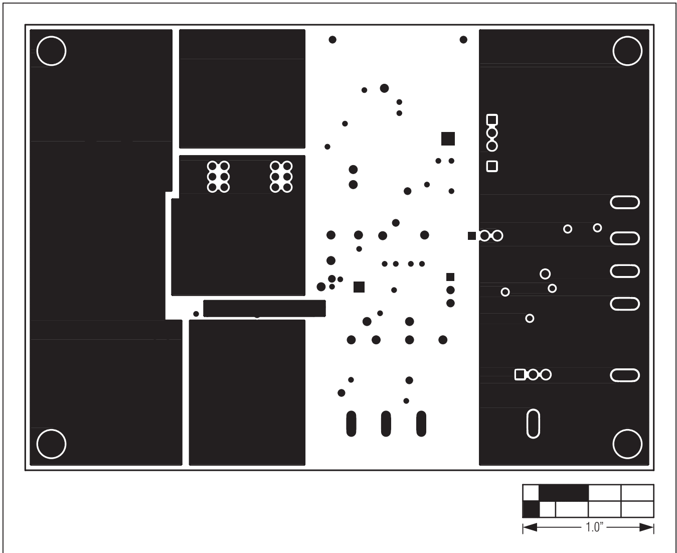
Figure 5. MAX5977A EV Kit PCB Layout—Inner Layer 3
