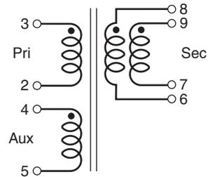
Secondary windings to be connected in parallel on the PCB.
