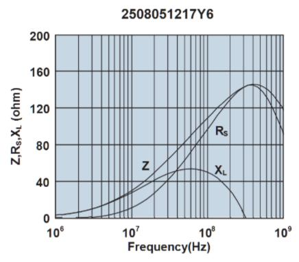
Impedance, reactance, and resistance vs. frequency.
