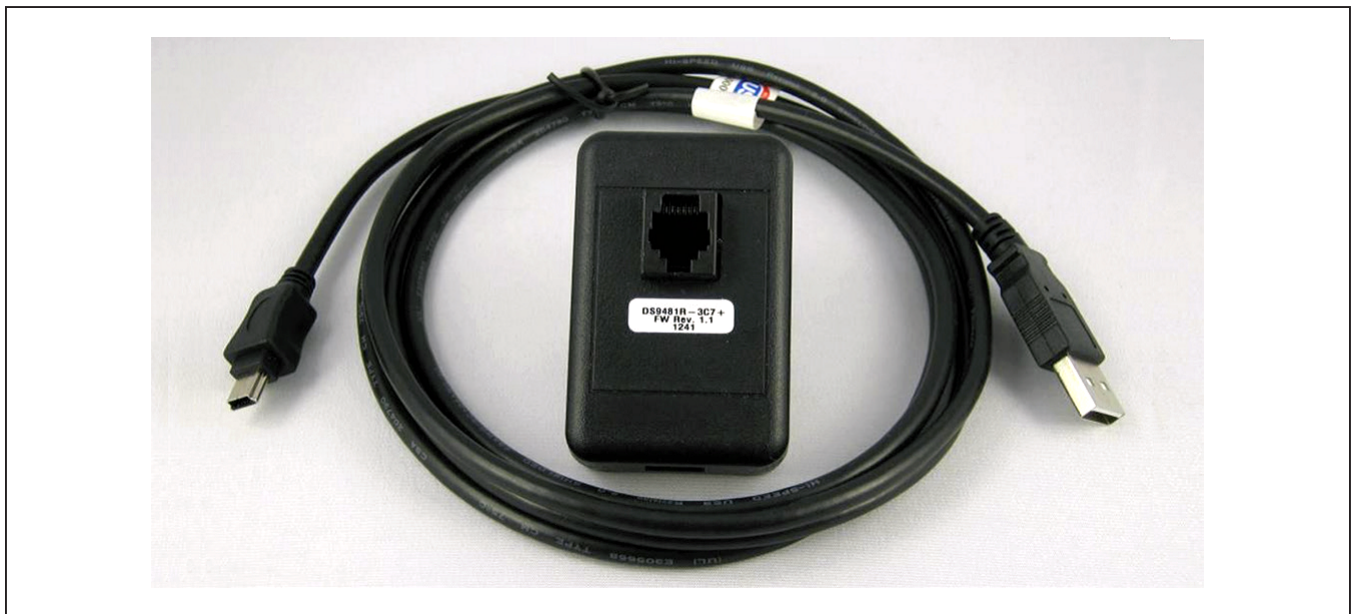
Figure 2. DS9481R-3C7+ USB-to-1-Wire/iButton Adapter
