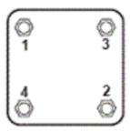
4. Apply no-flux solder to each pin of the TGA2625-CP. The component leads should be manually soldered, and the package cannot be subjected to conventional reflow processes. The use of no-clean solder to avoid washing after soldering is recommended.
