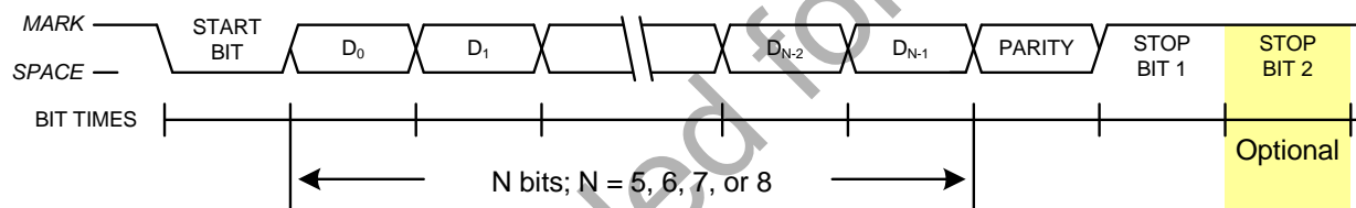
Figure 21.3. UART1 Timing With Parity
