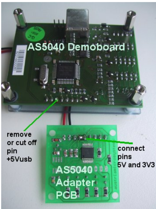
Figure 9: configuring the Adapter PCB for 3.3V operation
