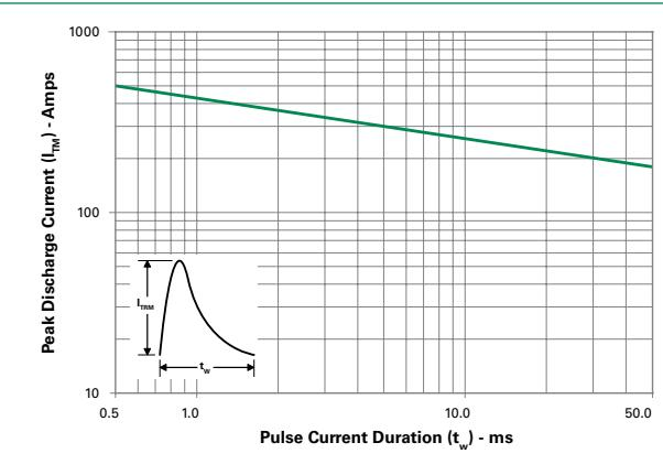
**Figure 9: Peak Capacitor Discharge Current Derating**
