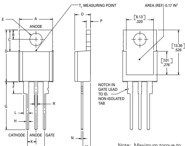
Note: Maximum torque to be applied to mounting tab is 8 in-lbs. (0.904 Nm).
