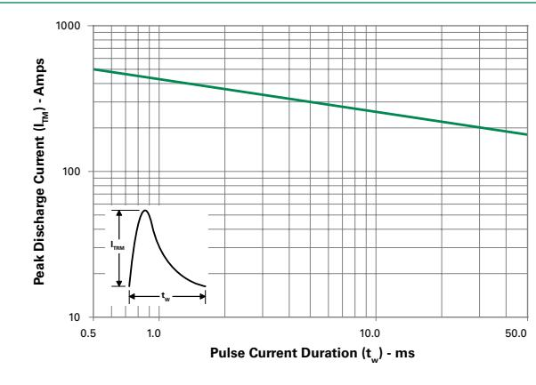
**Figure 9: Peak Capacitor Discharge Current Derating**
