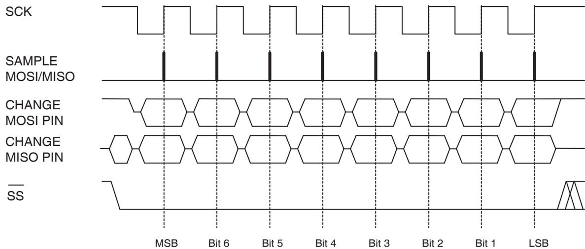
Figure 6-2. Data Byte Exchange – Timings
