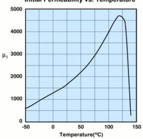
Measured on a 17/10/6mm toroid at 100kHz.
