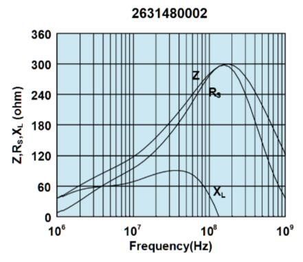
Impedance, reactance, and resistance vs. frequency.
