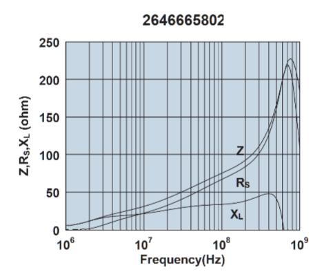
Impedance, reactance, and resistance vs. frequency.
