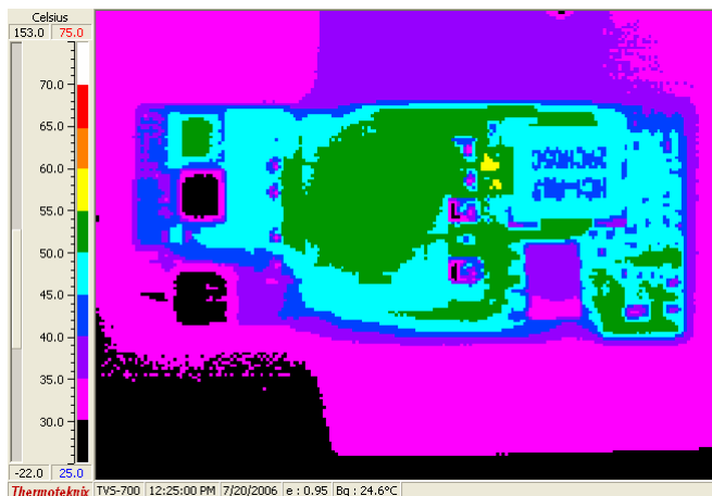
Figure 6. Temp Data (48Vin, 20A, 25°C, 200LFM airflow – front)
