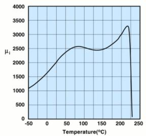
Measured on an 18/10/6mm toroid at 100kHz.
