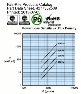
Measured on an 18/10/6mm toroid using the Clarke Hess 258 VAW at 100°C
