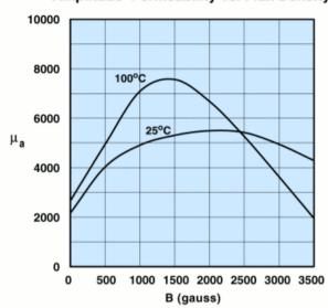
Measured on an 18/10/6mm toroid at 10kHz.
