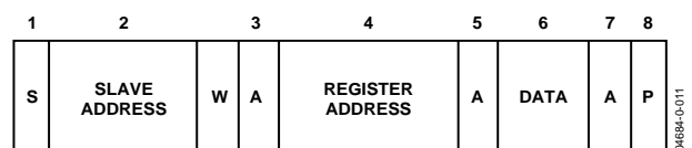
Figure 11. Single-Byte Write to a Register
