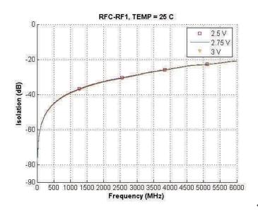
Figure 12. Isolation: RFC-RF1@ 2.75V
