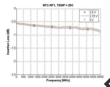
Figure 8. Insertion Loss: RFC-RF1@ 2.75V
