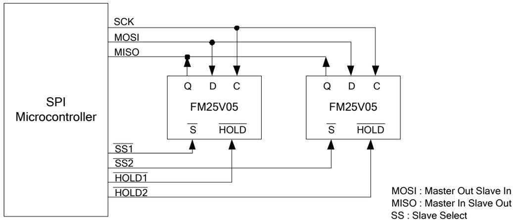
**Figure 3. 1Mbit (128KB) System Configuration with SPI port**
