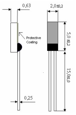
Polynomial of a nickel resistor in accordance with DIN 43760:  $R(\vartheta) = R_0 x (1 + 5,481 x 10^{-3} x \vartheta + 6,650 x 10^{-6} x \vartheta^2 + 2,805 x 10^{-11} x \vartheta^4 + 2,000 x 10^{-17} x \vartheta^6)$
