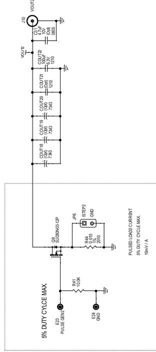
PWM ENABLE CIRCUIT FOR NON-THREE STATE COMPATIBLE DRMOs
