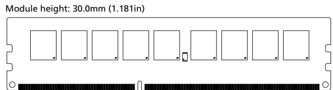
Figure 2: 240-Pin UDIMM (MO-269 R/C D1) PCBs 1483 & 1568
