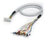
Assembled, shielded round cable with a 16-pos. socket strip and an open end. At the open end, the wires are labeled 1 to 16 and are fitted with ferrules, shield connection at open end, cable length: 27 m
