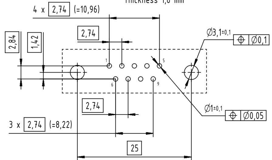
Connector retention and insertion forces on PC-Board: 25 N / 80 N
