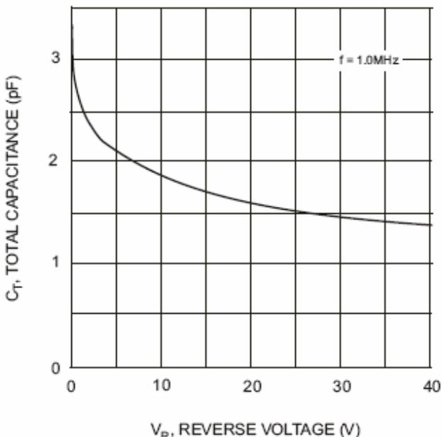
Fig. 3 Typical Capacitance
