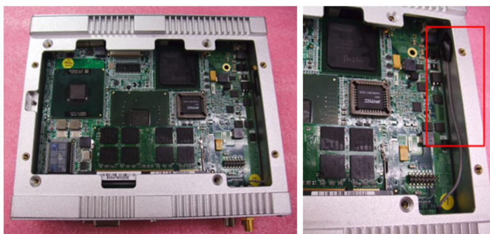
Figure 5.4 GPRS/EDGE SMA cable internally
