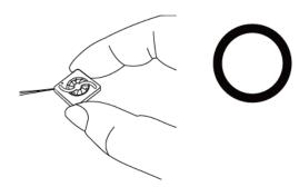
Don't pull fan with lead wires.
