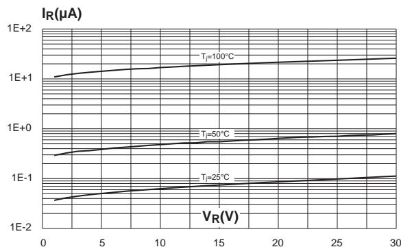
**Figure 4. Reverse leakage current versus junction temperature**
