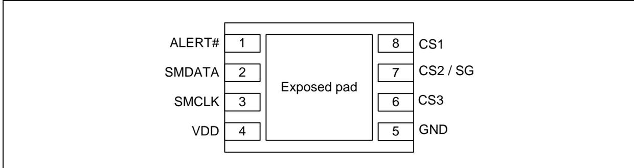
Figure 1.1 CAP1293-1 Pin Diagram (8-Pin 2mm x 3mm TDFN)
