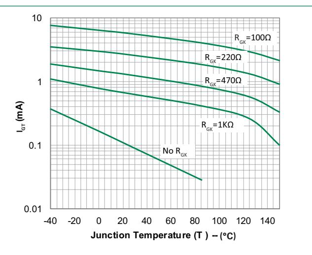
**Figure 12: Typical DC Holding Current with  $R_{GK}$  vs. Junction Temperature (Sensitive SCR)**
