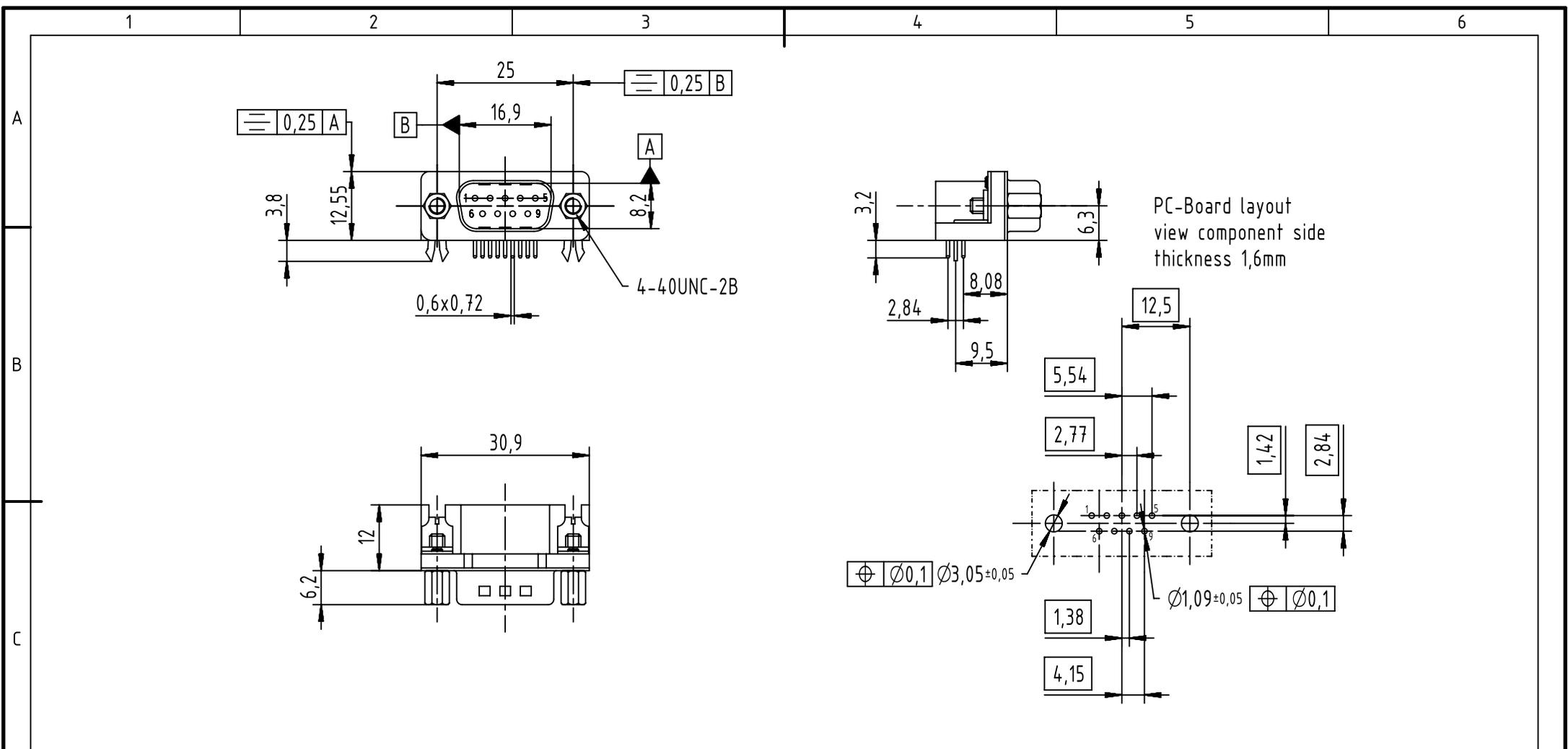
Connector insertion force on PCB = maxi 80N
