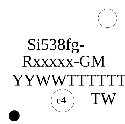
Figure 12.1. Si5381/82 Top Marking
