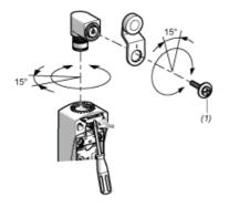
(1) Tightening torque (Min: 1) (Max: 1.5)
